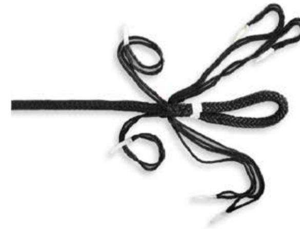
Remove tape wrap at Mark "A" and gently but firmly pull on each of the strand pairs so Mark "A" is now snug up to the base of the eye. (Mark B) Now complete two (2) more sets of tucks with each tapered strand pair. Be sure to tuck each strand pair down the same crown strand line - try to keep twist in each pair, and continually remove slack from each strand pair after tucking. (Fig. 5 & 6)
