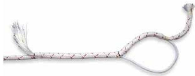
Use masking tape and overlap each wrap of tape as little as possible. After taping, roll the taped section between your hands to smooth the taped area. (Fig. 6)
